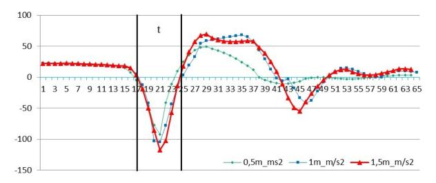
Figure 2. Typical curve acceleration of a head on contact with a ball with vertical velocity 3.13 m·s-1 (green curve), 4.43 m·s-1 (blue curve) a 5.43 m·s-1 (red curve)
