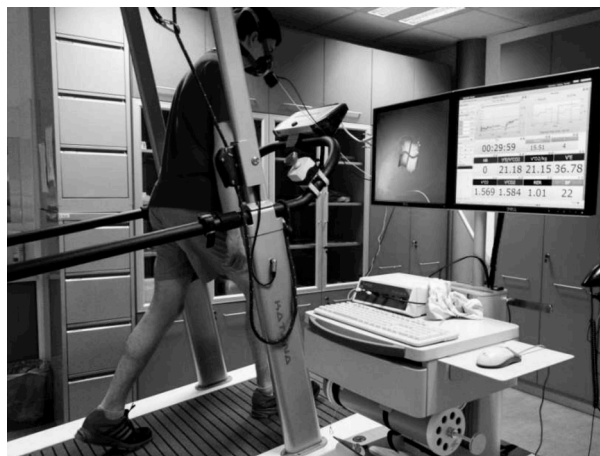
Figure 1. One of participants during test protocol (3 km/h and +12 % inclination of treadmill)
