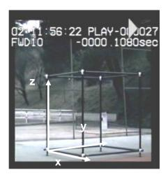
Figure 2. Calibration Object
