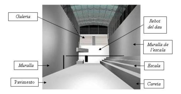
Figure 1. Parts of valencian ball trinquete.
