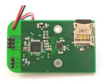
Figure 1. Accelerometer and gyroscope used for measuring
