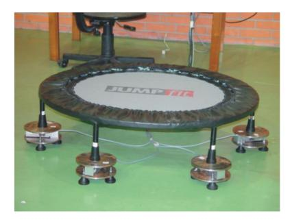
Figure 1. Rebound exercise mini-trampoline with attached load cells
