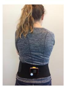
Figure 1. Subject wearing the IMU system mounted on a neoprene belt. The belt was placed at the L4/L5 level and a retroreflective marker was attached to the bottom left corner.
