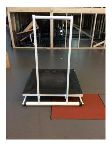
Figure 2. The trampoline was placed in the middle of the force plate with the handle in front of the subject. Subjects began behind the trampoline and then stepped on to perform the jump.
