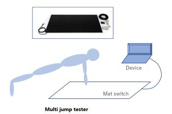
Figure 1. Multi-jump tester utilized for push up jump and countermovement push up assessments.
